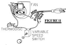
*10.* Bring out any slack in the blower cord. Place the cord into the split strain relief bushing, just at the point where the cord enters the slot. Clamp the two pieces together and insert the bushing securely into the slot.
