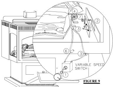
**6.** Connect one bare lead of wire **(B)** to the **white** wire of the speed switch using a nut connector. Connect the other end to the bare lead wire of the blower cord using a nut connector.
